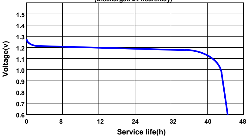
DISCHARGE CHARACTERISTICS AT 100Ω 20°C 60%RH (Discharged 24 hours/day)
