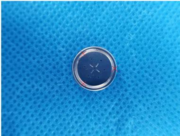
Electrostatic Discharge Test points
