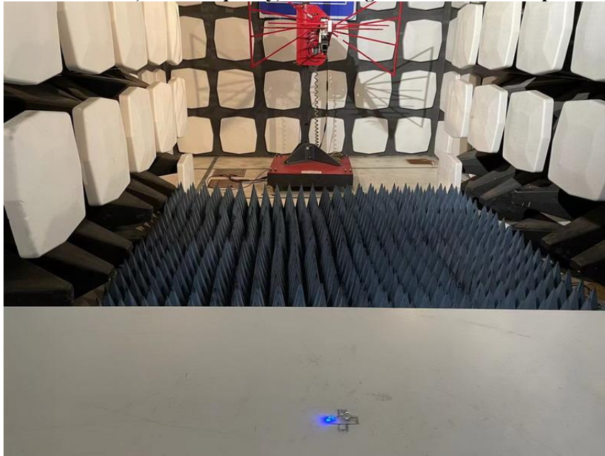
Radiated, radio-frequency, electromagnetic field Test Set Up
