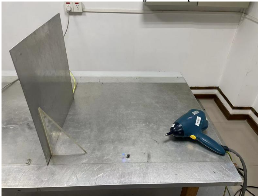
Electrostatic Discharge Test Set Up
